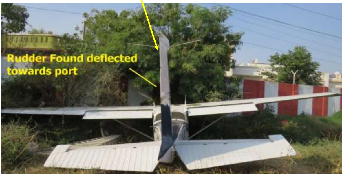
Image 37. Rudder found deflected towards port side
