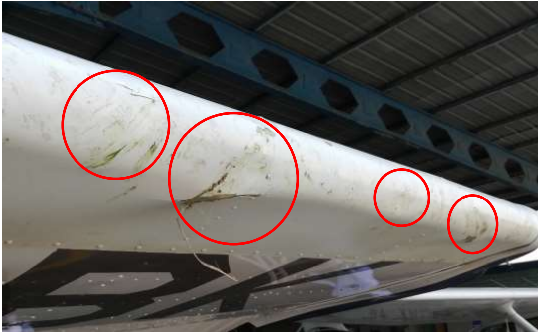
Image 3. Damages on Left Wing leading edge (Outboard)
