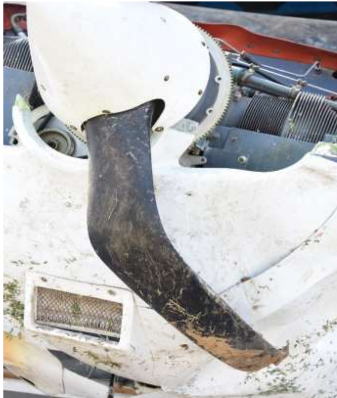
Image 1. Propeller blade found bent backwards
