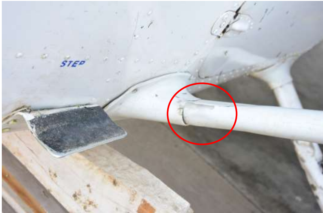
Image 19. Dent on LH wing strut
