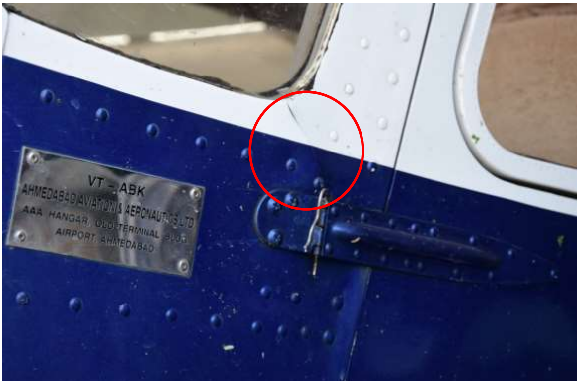
Image 7. Skin found bent above the upper hinge LH door
