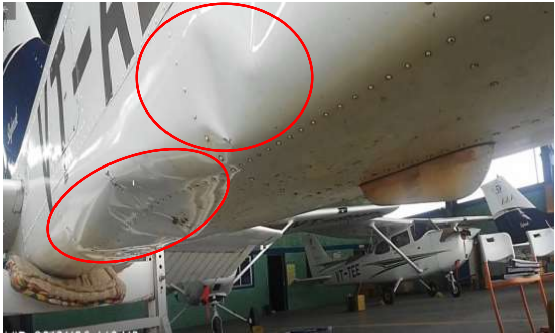
Image 8. Dents in fuselage RH side
