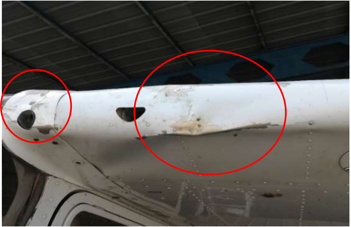
Image 4. Damages on Left Wing leading edge (Inboard)
