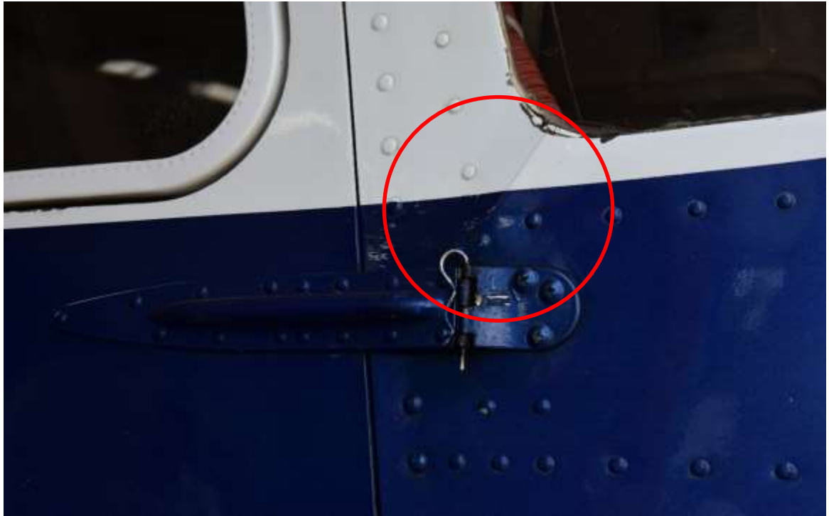
Image 6. Skin found bent above the upper hinge RH door
