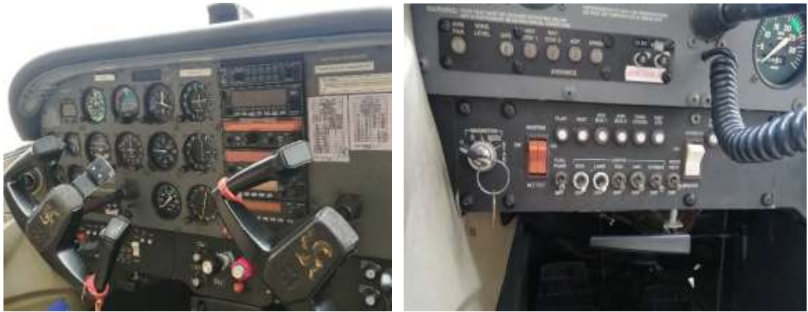
Image 34. All the switches in cockpit were in OFF/Pushed IN position.
