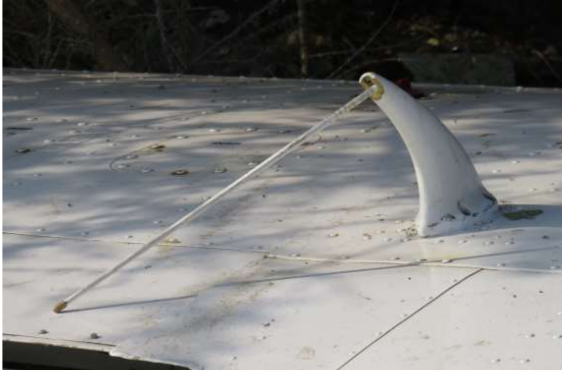
Image 12. Broken LH VHF Antenna
