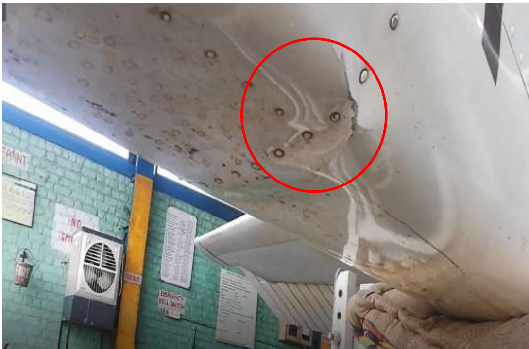
Image 9. Dent in Fuselage LH lower surface
