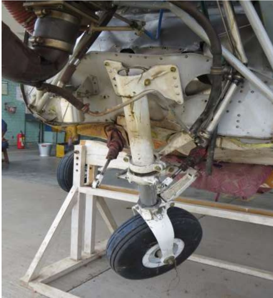
Image 17. Nose Wheel bent backwards
