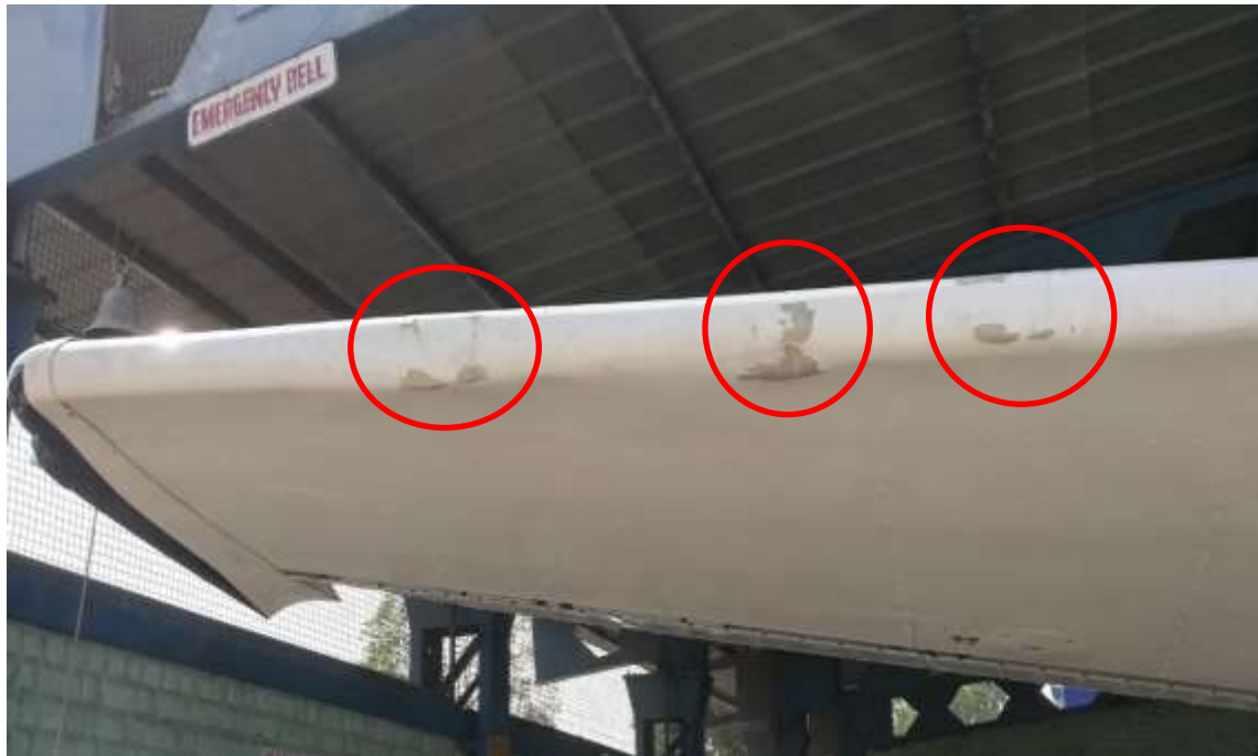
Image 5. Damages on Right Wing leading edge
