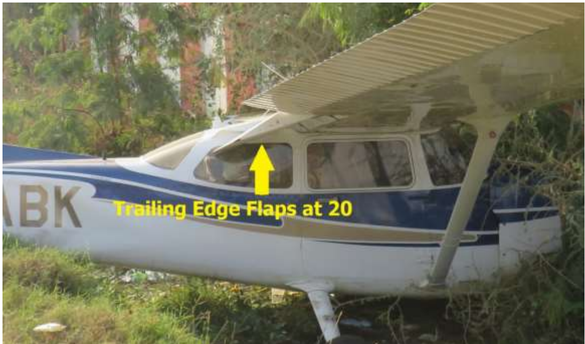
Image 35. Trailing Edge Flaps at 20° Position
