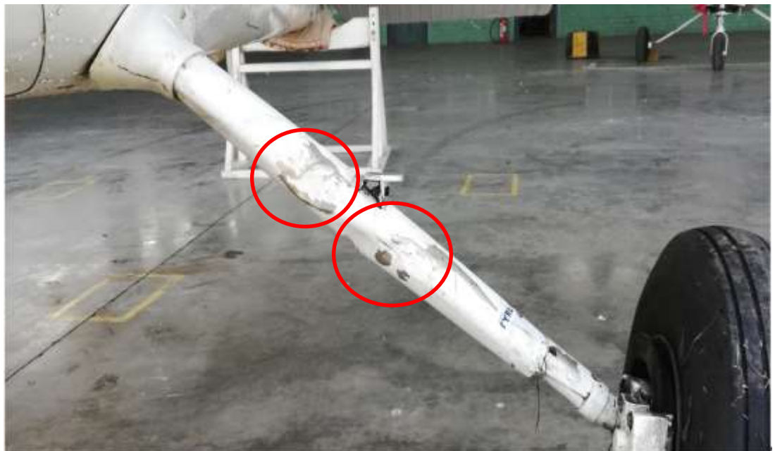
Image 11. Dents in LH main wheel strut fairing
