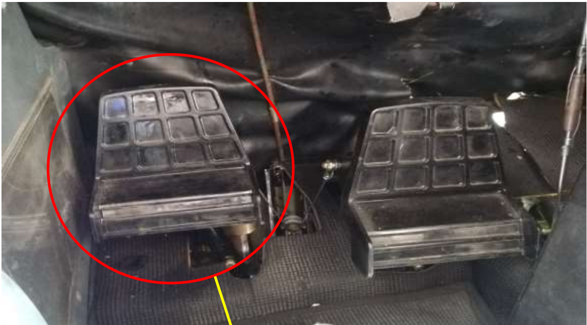
Image 36. Rudder pedal Position in cockpit (Left pedal pushed in)
