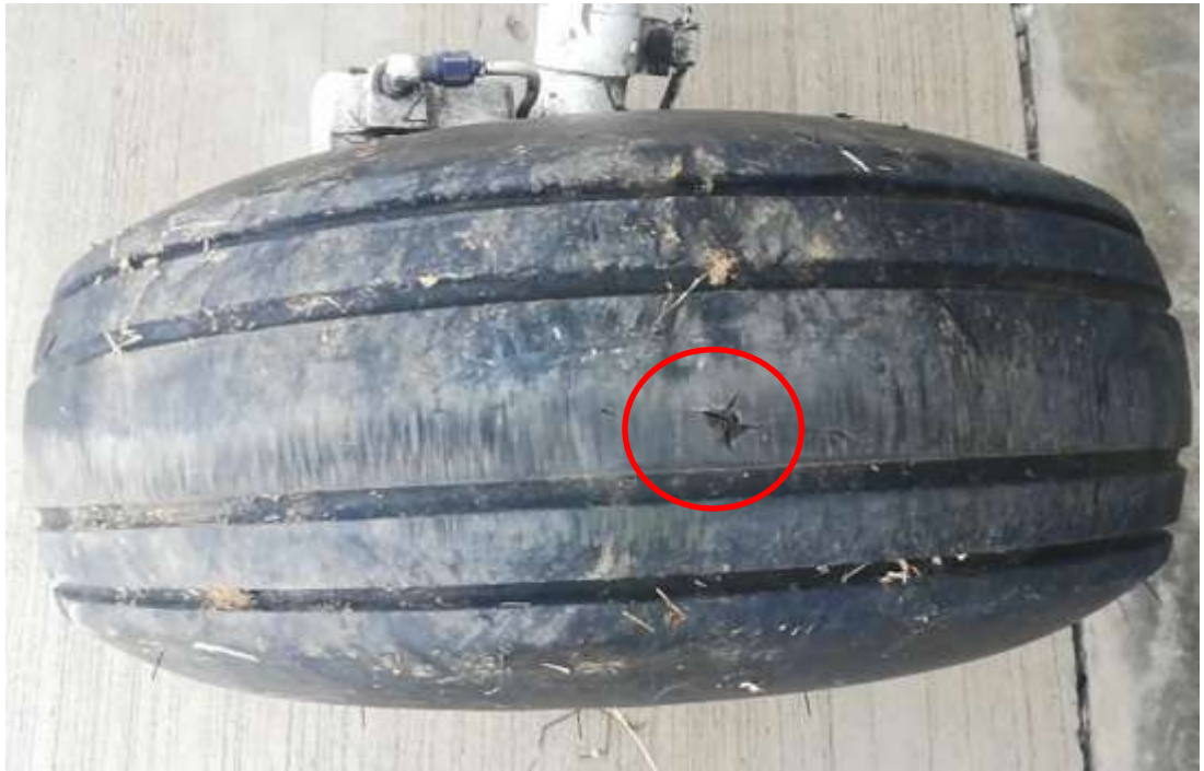
Image 10. Cut Mark on LH tyre
