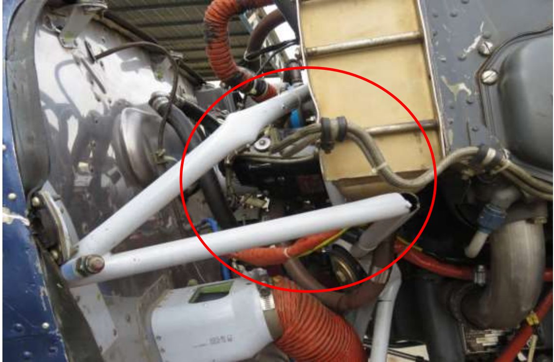
Image 15. Broken Engine Mount
