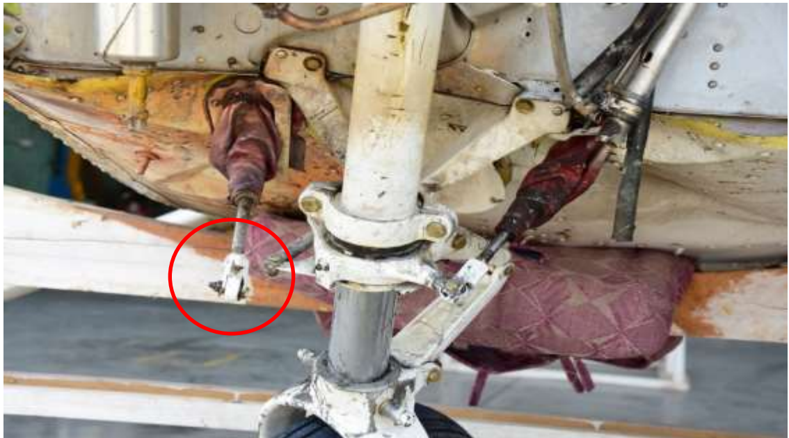
Image 16. Broken RH side steering rod eye end
